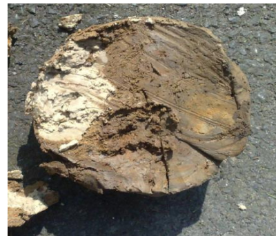
Figure 7 – Borehole Core - showing Bentonite Plugging.
