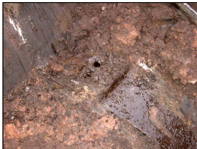
Plate 2 - Contaminated soils with free phase hydrocarbon – typical of the contamination throughout the site.
