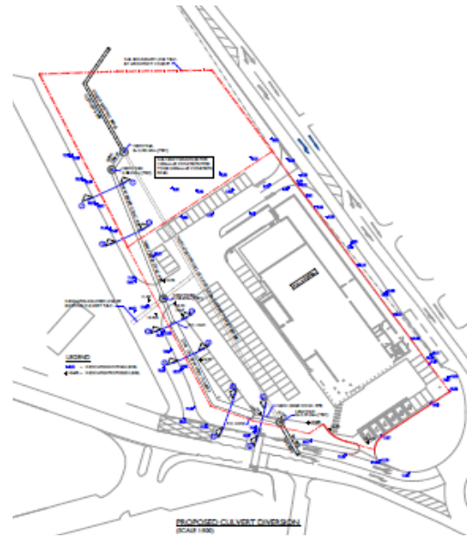
Figure 4 – Location of Realigned Culvert
