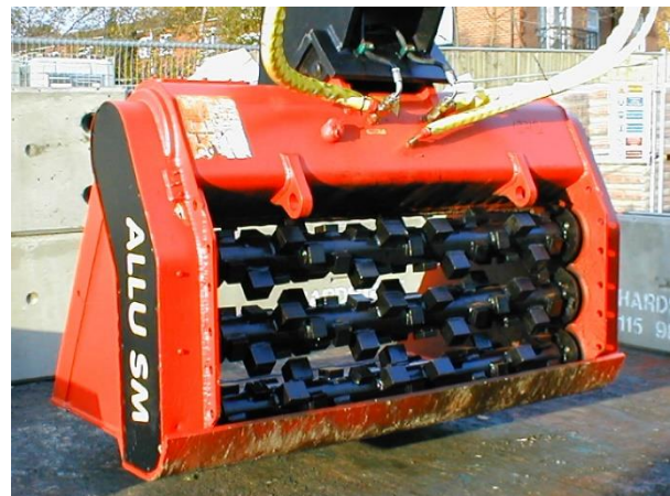
Figure 3 – Allu bucket used for mixing operations
