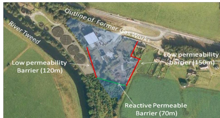
Plate 5 – The Installed Soil Mixed Barrier System for the Eshiels Project
