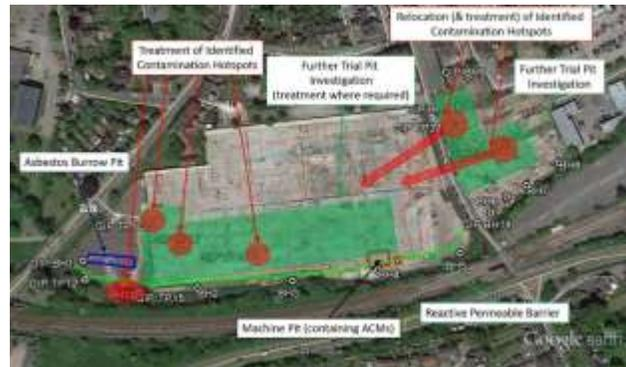
The remediation scheme was implemented under the auspices of Envirotreat's Mobile Treatment Permit authorised by the Environment Agency. The treatment process is licensed as a waste recovery operation enabling reuse of treated [recovered] materials on-site (as a substitute for imported fill) in accordance with the Materials Management Plan [MMP] for the site.
