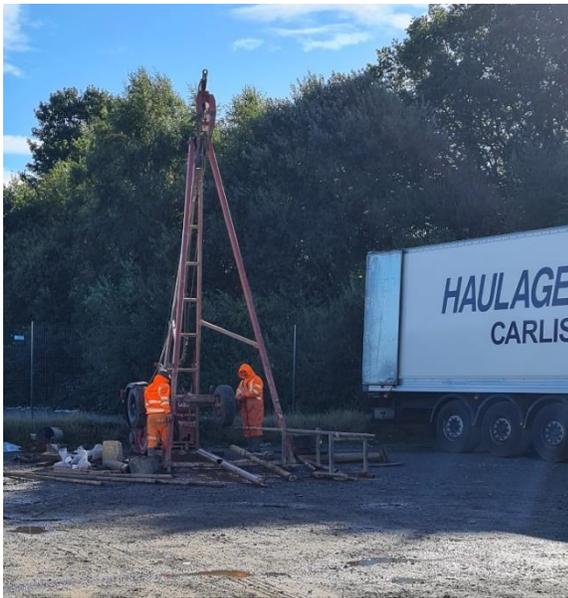
In-situ penetration tests, comprising CPTs, were completed at 1m intervals in each borehole in accordance with BS EN ISO 22476-3:20059.
